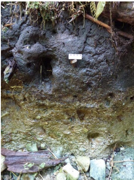
Image 7: Peat deposit overlying glacial deposit (till), West Lake Forest Access Road (WLFAR). Scale divided into seven one-centimetre sections.
